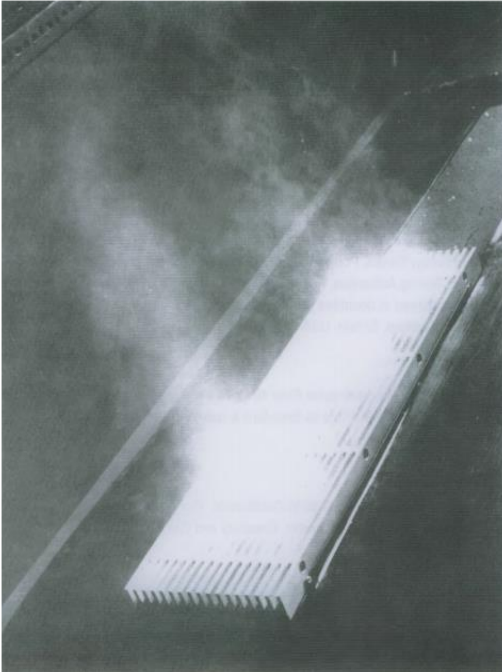
Installed computer floor grille in laboratory for testing. Floor is painted black to facilitate witnessing smoke pattern.
